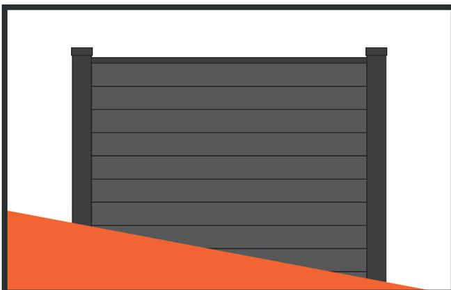
**Installation Top Tip** - If you are installing the fencing on a gradient or slope, mitre (cut) the respective Fence Boards to the desired angle and length.
