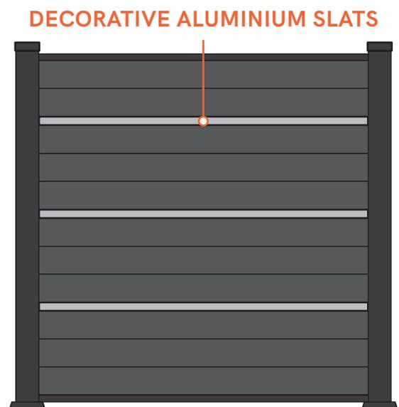
This configuration, based on standard measurements of 1800mm (W) x 1890mm (H), will have 11 Fence Boards and 3 Decorative Aluminium Slats (1 Kit).
